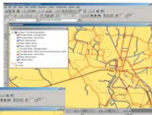
A thematic display of roadway functional classifications – principal artery, interstate, minor artery, and so forth – has been dynamically segmented onto the roadway network.
