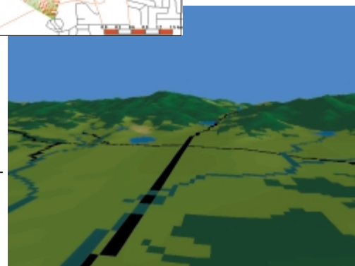
A 3D Perspective view is created by draping the contents of a MapView window over the triangulated elevation model.
