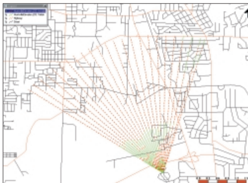
A Visibility Fan shows the visible or hidden portions of multiple Line-of-Sight rays from a specific viewpoint.
