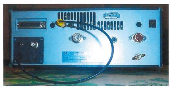
Now, the AN-1 is powered only when the IC-R8500 is on so needs no specific power supply.
